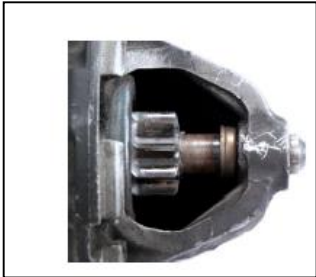
Meshing: Blue Shaft Worn / Broken Teeth
