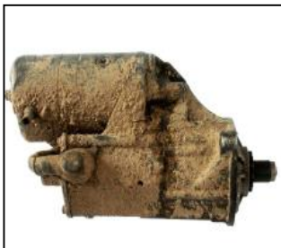
Contamination: Sand / Dirt etc.
